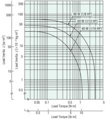
Speed at Output Shaft: 100 r/min Gear Ratio 18:1 at 60 Hz
