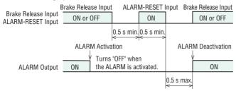
It is also possible to deactivate the alarm by turning off the power supply and turning it on again. Turn off the DC or AC power supply, and turn all input signals "OFF" before turning it on again.
