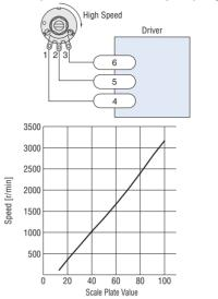
External Speed Potentiometer Scale—Speed Characteristics (Representative values)
