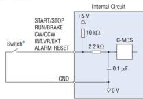
\*Use a switch capable of opening/closing the current flow at 5 VDC, 1 mA maximum.
