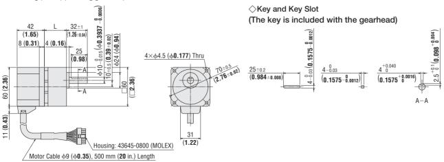
lacksquare Enter the gear ratio in the box ( $\Box$ ) within the model name.
