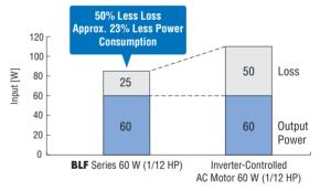
Brushless motors, which incorporate permanent magnets in the rotor, generate little secondary loss from the rotor.
