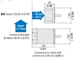
The compact yet powerful motor incorporates permanent magnets in the motor rotor. Compared with an AC motor having a frame size of 90 mm (3.54 in.), a brushless motor of the same specifications is 75 mm (2.95 in.) shorter and offers 1.3 times more output. The compact motor structure lets you downsize your equipment.
