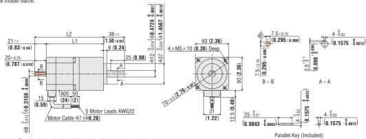
• These dimensions are for the double shaft models. For the single shaft models, ignore the orange (\_\_\_\_\_) areas.
