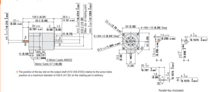
• These dimensions are for the double shaft models. For the single shaft models, ignore the orange (\_\_\_\_\_) areas.
