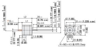
\* The length of machining on the double shaft model is 15±0.25 (0.591±0.010).
