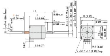
\* The length of machining on the double shaft model is  $10\pm0.25$  (0.394 $\pm0.010$ ).
