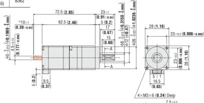
\* The length of machining on the double shaft model is  $10\pm0.25$  (0.394 $\pm0.010$ ).
