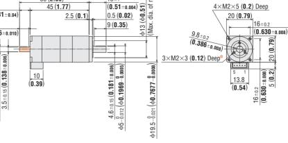
\* The position of the machining on the output shaft  $[\phi 5 (\phi 0.1969)]$  relative to the screw holes position on a maximum diameter of  $\phi$ 13 ( $\phi$ 0.51) on the rotating part is arbitrary.
