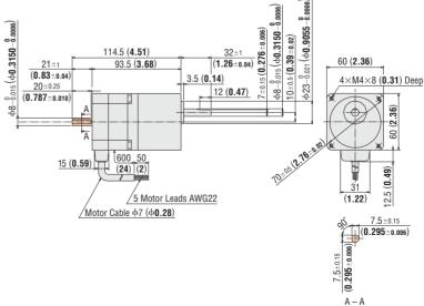
• These dimensions are for the double shaft models. For the single shaft models, ignore the orange (\_\_\_\_\_) areas.
