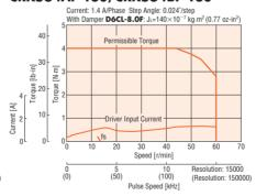
• The pulse input circuit responds to approximately 500 kHz with a pulse duty of 50%.
