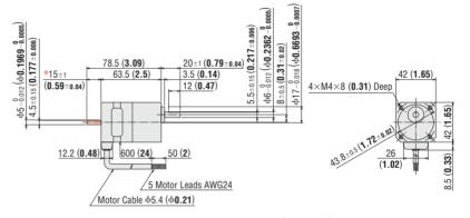
\* The length of machining on the double shaft model is 15±0.25 (0.591±0.010).
