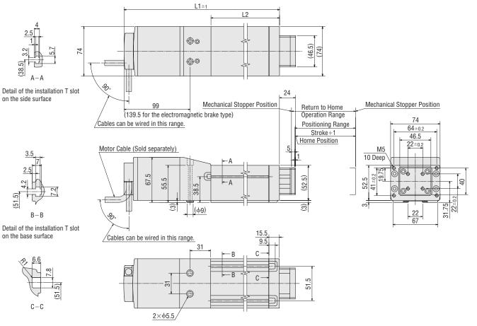
Cylinder Model: EZAM6D A, EZAM6E A, EZAM6D C, EZAM6E C (Without electromagnetic brake) EZAM6D MA, EZAM6E MA, EZAM6D MC, EZAM6E MC (With electromagnetic brake)
