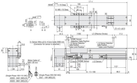
\* The settings "55," "10" and "112" indicate the recommended mounting positions of the -LS sensor, HOME sensor and +LS sensor, respectively. Sensors and a shield plate can also be installed on the opposite side.
