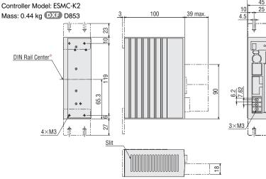
\*The center of the DIN rail when a DIN rail mounting plate (PADPO1, sold separately) is used for installation.
