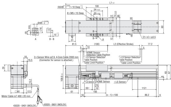
\* The settings "55," "10" and "112" indicate the recommended mounting positions of the -LS sensor, HOME sensor and +LS sensor, respectively. Sensors and a shield plate can also be installed on the opposite side.
