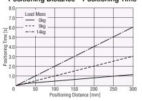
• The positioning time in the graph does not include the settling time. Use a settling time of 0.15 s as a reference. (Settling time is adjustable by speed filter function.) • The starting speed should be 6 mm/s or less.
