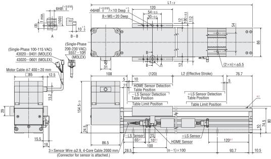
\*1 The settings "65," "10" and "120" indicate the recommended mounting positions of the -LS sensor, HOME sensor and +LS sensor, respectively. Sensors and a shield plate can also be installed on the opposite side.
