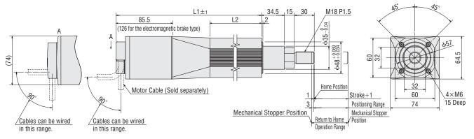
Cylinder Model: EZCM6D A, EZCM6E A, EZCM6D C, EZCM6E (Without electromagnetic brake) EZCM6D MA, EZCM6E MA, EZCM6D MC, EZCM6E MC (With electromagnetic brake)
