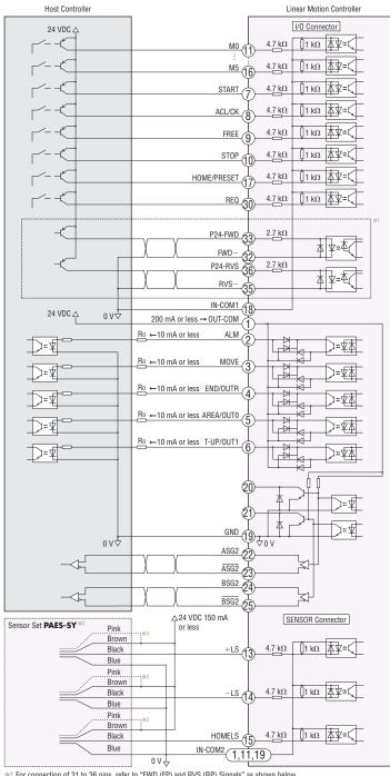
\*1 For connection of 31 to 36 pins, refer to "FWD (FP) and RVS (RP) Signals" as shown below. \*2 An accessory sensor set is also available (sold separately.)
