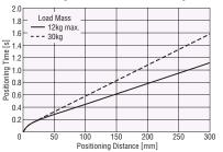
The positioning time in the graph does not include the settling time. Use a settling time of 0.15 s as a reference. (Settling time is adjustable by speed filter function.)
