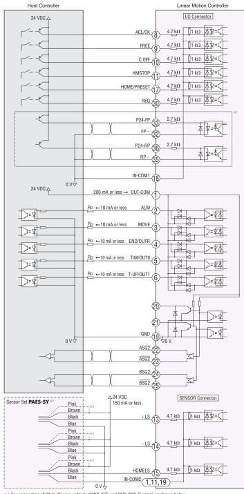
\*1 For connection of 31 to 36 pins, refer to "FWD (FP) and RVS (RP) Signals" as shown below. \*2 An accessory sensor set is also available (sold separately.) \*3 Connect this line if the normally closed (NC) logic is used.
