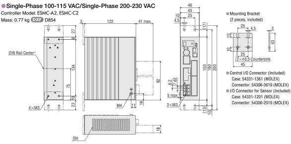
\*The center of the DIN rail when a DIN rail mounting plate (PADPO1, sold separately) is used for installation.
