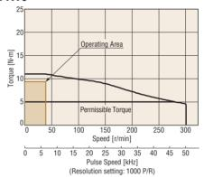
PN geared type can operate inertia load up at starting/stopping to acceleration torque less than maximum torque.
