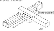
Ly: Center of gravity of load [mm] m: Mass of load [kg]
