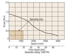
Select a motor for which the operating area indicated by operating speed and required torque falls within the pullout torque of the speed – torque characteristics.
