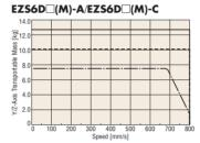
\*For X-axis, the maximum speed read from the graph is limited by the stroke. Check the maximum speed for each stroke in EZSII Series products.
