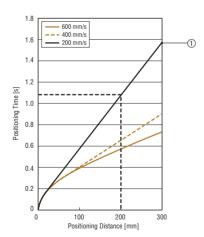
The above graph shows that the load can be positioned over 200 mm within 1.5 second.
