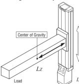
Lz: Center of gravity of load [mm] m: Mass of load [kg]
