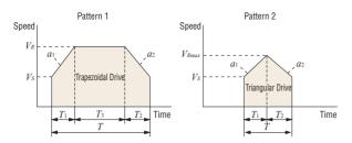
V<sub>Rmax</sub>: Calculated maximum speed of triangular drive [mm/s]
