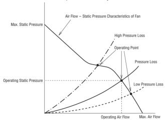
Air Flow - Static Pressure Characteristics
