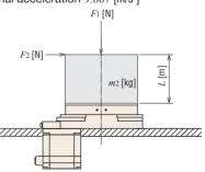
Thrust load [N]  $F_S = F_1 + m_2 \times g$ Moment load [N·m]  $M = F_2 \times (L + a)$
