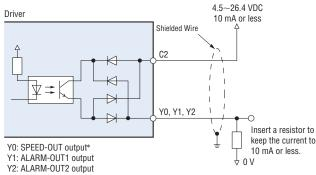
\*Supply a current of 5 mA or more to the SPEED-OUT output.
