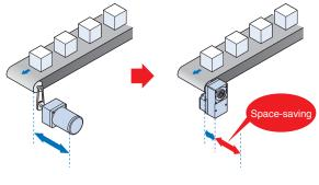
[For Three-Phase Motor and Parallel Shaft Gearhead]
