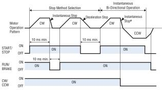
\* Changing the direction while the motor is running will cause the motor to stop instantaneously and then change its direction.
