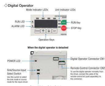
External Voltage Select Switch To set speeds using external DC voltage, set this switch to 5 V or 10 V in accordance with the voltage supply used
