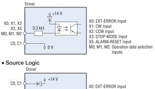
X1: CW Input X2: CCW Input X3: STOP-MODE Input X5: ALARM-RESET Input M0, M1, M2: Operation data selection inputs
