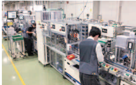
Motor assembly line collaborated with automation and human skills
