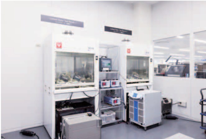
Locked rotor test (in Product Safety Testing Laboratory)
