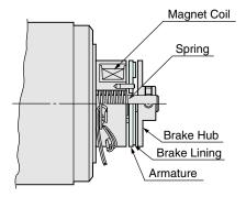
The figure above provides an example of the electromagnetic brake motors structure.
