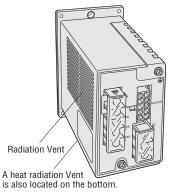
Mount the control unit 0.98 in. (25mm) or more away from the housing and other equipment inside the housing in the horizontal direction, and 1.97 in. (50mm) or more away in the vertical direction.
