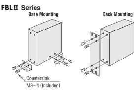
To improve ventilation, mount the driver in an upright position as shown in the figures above.
