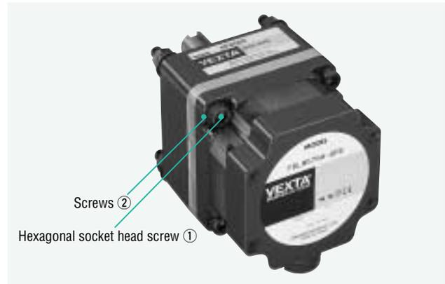
Install the motor and gear combination using the four hexagonal socket head screws ①.
