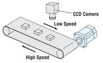
$\alpha_{\text{STEP}}$  is well-suited to applications where smooth movement or stability is required, such as where a camera is used to monitor the quality of a product.
