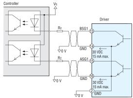
Circuits for use with 30 VDC, 15 mA maximum. A counter or similar device can be connected to monitor the position of the motor. The pulse resolution is the same as the motor resolution at the time of power-on.
