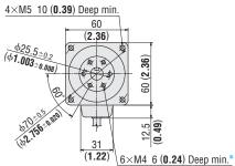
\*The position of the key slot on the output shaft [ $\phi$ 12 ( $\phi$ 0.4724)] relative to the screw holes on a maximum diameter of  $\phi$ 33.5 ( $\phi$ 1.32) on the rotating part is arbitrary
