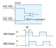
To monitor the motor position, connect these signals to a counter, etc. The pulse resolution is the same as the motor resolution at the time of power-on.
