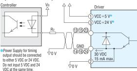
Circuits for use with 30 VDC, 15 mA maximum.
