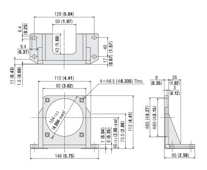
This installation plate is convenient for installing the driver of *Xstep* AS Series on DIN rails with ease.
