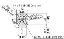
\*The position of the key slot on the output shaft [φ10 (φ0.3937)] relative to the screw holes on a maximum diameter of φ26.5 (φ1.04) on the rotating part is arbitrary.
