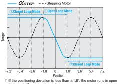
loop mode like a stepping motor. (2)If the positioning deviation is  $\pm 1.8^{\circ}$  or more, the motor runs in closed loop mode and the position is corrected by exciting the motor windings to generate maximum torque based on the rotor position.
