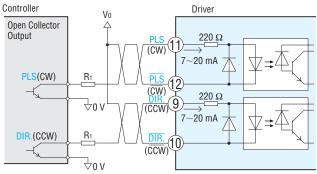
•The colored characters indicate signals under the 1-pulse input mode, while the black characters indicate signals under the 2-pulse input mode.
