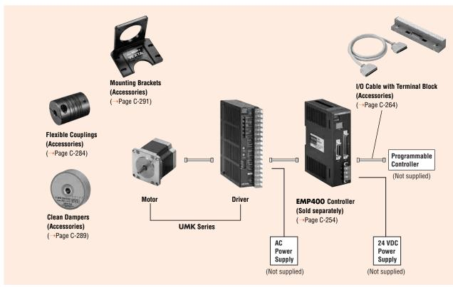
An example of a single-axis system configuration with an EMP400 series controller.
