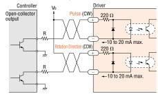
The characters indicate signals under the 1-pulse input mode, while the characters in parentheses indicate signals under the 2-pulse input mode. **Note:**
