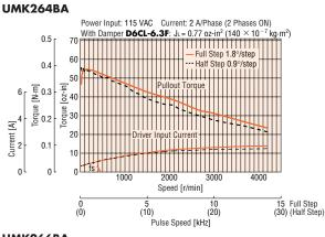
Power Input: 115 VAC Current: 2 A/Phase (2 Phases ON) With Damper **D6CL-6.3F**:  $J_L = 0.77$  oz-in<sup>2</sup> (140  $\times 10^{-7}$  kg·m<sup>2</sup>)
