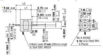
\* The length of machining on double shaft model is **0.591**±**0.010** (15±0.25).
