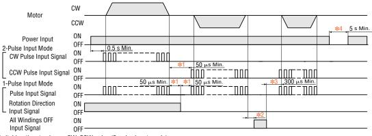
\*1 Switching time to change CW, CCW pulse (2-pulse input mode)
