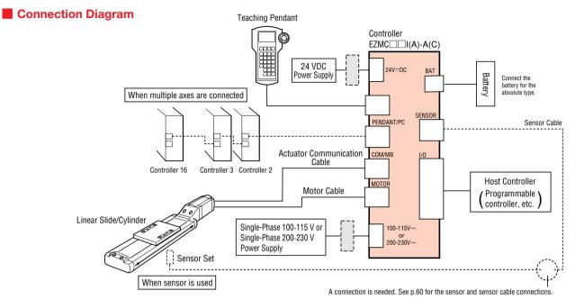
For the section indicated by broken line, see following "Connection Example of Power System and Emergency Stop System".
