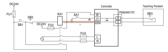
• FU1: Ground-fault protection fuse (500 mA)
