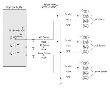
•V1 must be between 5 VDC and 24 VDC. The current must be 100 mA or less. If the current exceeds 100 mA, connect an external resistance R.
