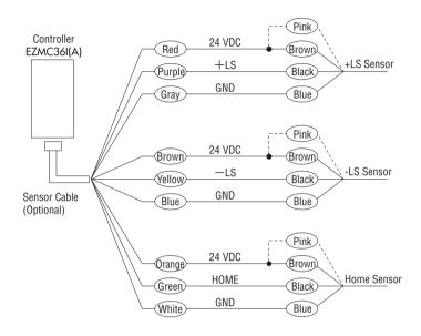
•The 24 VDC output from the controller is used to drive the sensors.
