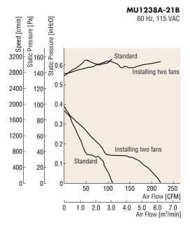
Fig. 6 Changes in fan characteristics of static pressure and amount of air flow
