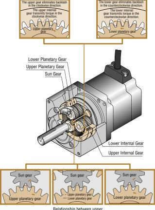
Relationship between upper and lower planetary gears
