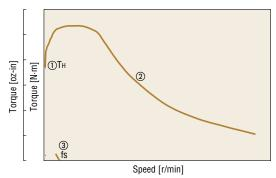
Speed vs. Torque Characteristics
