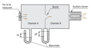
Fig. 4 Double-chamber Measuring Device
