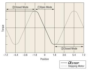
Angle vs. Torque Characteristics
