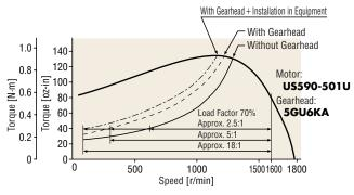
Due to the aforementioned advantage of heat dissipation, when a motor is installed in equipment it can often be operated at variable speeds with a speed ratio of 18:1, as long as the load factor does not exceed 70%.
