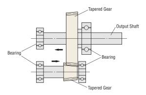
Structure of **TH** gear's final stage
