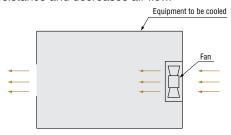
Fig. 1 Flow Path with Low Air Flow Resistance
