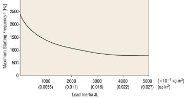
Load Inertia vs. Starting Frequency Characteristics
