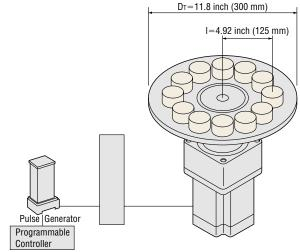
Diameter of index table:  $D_T = 11.8 \text{ inch (300 mm)}$  Index table thickness:  $L_T = 0.39 \text{ inch (10 mm)}$  Thickness of work:  $L_W = 1.18 \text{ inch (30 mm)}$  Diameter of work:  $D_W = 1.57 \text{ inch (40 mm)}$  Material of table and load: Iron [density  $\rho = 4.64 \text{ oz/in}^3$   $(7.9 \times 10^3 \text{ kg/m}^3)$ ] Number of loads:  $10 \text{ (one every } 36^\circ)$
