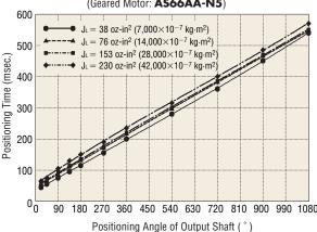
While the shortest positioning time of the motor changes significantly with the increase in load inertia, that of the geared motor shows little change. In other words, the geared motor is capable of driving a larger load inertia within the most consistent, shortest positioning time.
