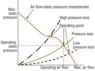
Air Flow-Static Pressure Characteristic
