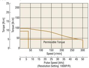
The total torque of the system is the sum of the load torque plus the acceleration torque. The total torque times the safety factor must not exceed the permissible torque.
