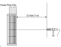
Fig. 9 Measurement of Fan Noise
