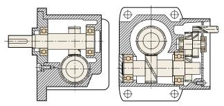
Structure of the Screw Gear
