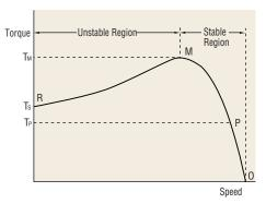
Under conditions of no load, the motor rotates at a speed close to synchronous rotation (O) . As the load increases, the motor's speed drops to a level (P) where a balance is achieved between load and motor torque (Tp).
