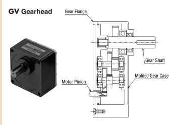
For use with general AC motors, many of which are fixed speed motors, the availability of various gear ratios suits a wide range of desired speeds. We support these motors with as many as 20 different gear ratios, ranging from 3:1 to 180:1.
