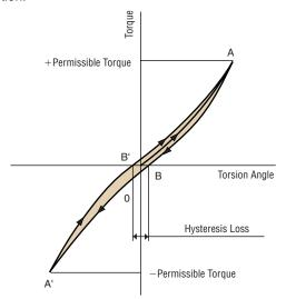
Torsion Angle and Torque Characteristics
