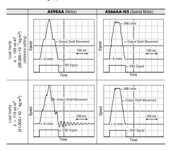
Even under the operating conditions that are optimized to reduce damping with a given load inertia, the damping characteristics of the motor will deteriorate with fluctuations in load inertia. For the motor it is therefore necessary to reset the operating conditions for optimal performance each time the load inertia fluctuates. On the other hand, the geared motor's damping characteristics change little with fluctuations in load inertia, thereby ensuring steady operation.
