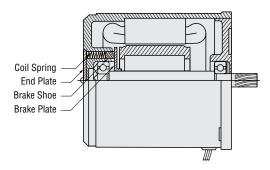
The brake mechanism is constructed as shown in the figure above. The coil spring applies constant pressure to allow the brake shoe to slide toward the brake plate. This mechanism provides a certain degree of holding brake force, but the force is limited due to the mechanism's structure, as described above. The brake force produced by the brake mechanism of an Oriental Motor reversible motor is approximately 10% of the motor's output torque.
