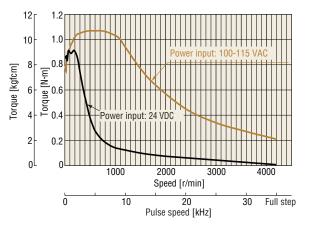
Comparison of the characteristics of AC input and DC input
