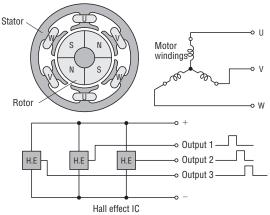
A Hall effect IC is used for the sensor's magnetic element. Three Hall effect ICs are placed within the stator, and send digital signals as the motor rotates.
