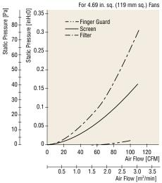
Fig. 7 Changes in Characteristics with Optional Parts
