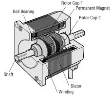
Motor Structural Diagram 1: Cross-Section Parallel to Shaft
