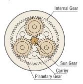
Cross Section of a PN Gear
