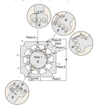
In other words, when excitation switches from phase A to B, the rotor rotates by 0.72°. As excitation shifts from phase A, to phases B, C, D and E, then back around to phase A, the stepping motor rotates precisely in 0.72° steps.
