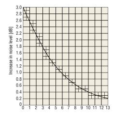
Fig. 10 Difference in Two Noise Levels
