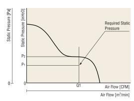
Fig. 3 Air Flow vs. Static Pressure Characteristics Curve
