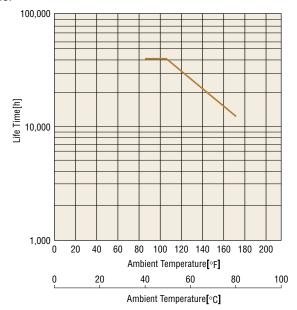
Fig. 12 Estimated Life Characteristics of the MU1238A Fan
