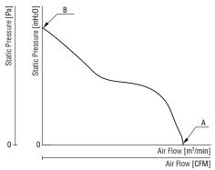
Fig. 14 Air Flow/Static Pressure Characteristics Curve
