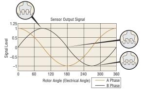
Output Signal of Rotor Position Sensor
