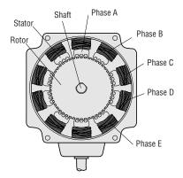
Motor Structural Diagram 2: Cross-Section Perpendicular to Shaft
