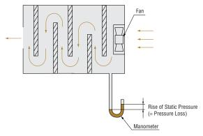
Fig. 2 Flow Path with High Air Flow Resistance
