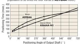
The geared motor is more effective in reducing the positioning time for a smaller positioning angle and a larger load inertia. The geared motor tends to achieve shorter positioning time in a wider range of positioning angles with a larger load inertia.
