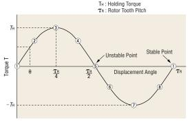
Angle vs. Torque Characteristics
