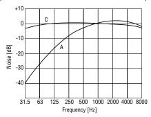
Fig. 16 Comparison of Sound-Pressure Level
