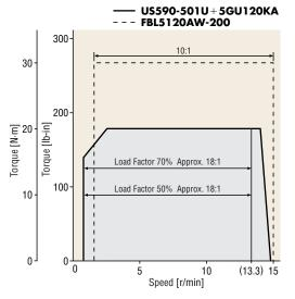
The maximum permissible torque of the **5GU120KA**, which has a gear ratio of 120:1, is 177 lb-in (20 N·m). The speed ratios at 50% and 70% load factors are shown in the table below:
