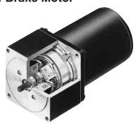
The photograph above shows the structure of the clutchbrake motor. When 24 VDC is not applied to either the clutch coil or brake coil, the output shaft can be rotated by hand.
