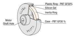
The clean damper, a viscous inertial damper is made of silicon gel encased in an airtight plastic package. Viscous inertia dampers are ideal for absorbing oscillation energy and shortening settling time.
