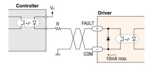
Keep the voltage between DC 5V and DC 30V.
