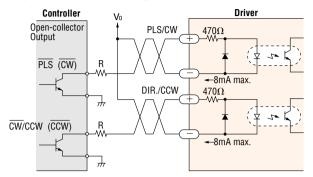
Keep the voltage between DC 5V and DC 12V.
