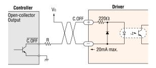
Keep the voltage between DC 5V and DC 24V.
