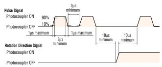
The shaded area indicates when the photocoupler diode is ON. The motor moves when the photocoupler state changes from ON to OFF as indicated by the arrow.
