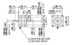
UMK266MAA (Single shaft) Motor Model: PK266MA Weight 1.55 lb. (Mass 0.7kg) UMK266MBA (Double shaft) Motor Model: PK266MB Weight 1.55 lb. (Mass 0.7kg)
