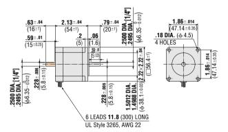
UMK268MAA (Single shaft) Motor Model: PK268MA Weight 2.21 lb. (Mass 1kg) UMK268MBA (Double shaft) Motor Model: PK268MB Weight 2.21 lb. (Mass 1kg)
