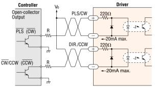
Keep the voltage between DC 5V and DC 24V.
