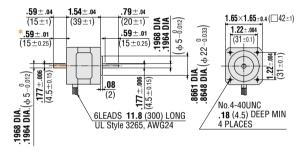
\* .59±.01(15±0.25) indicates the length of milling on motor shaft.
